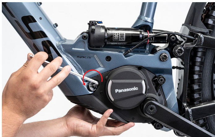
FIGURE 1: SCREW LOCATION AND ROTATION DIRECTION
