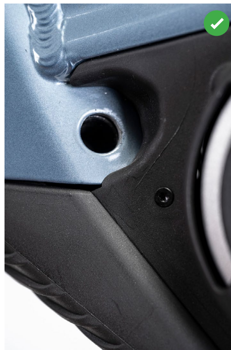
FIGURE 6: CHECK THE HOLE CONCENTRICITY IN THE FRAME AND THE BATTERIES
