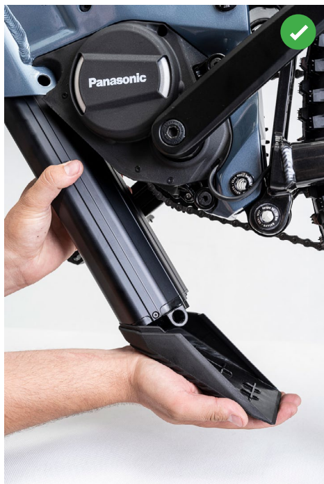
FIGURE 4: CORRECT BATTERY HOLDING
