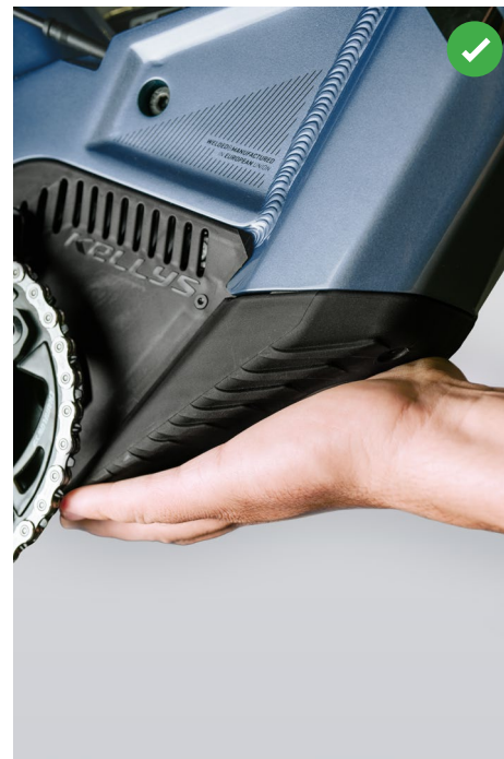
FIGURE 8: CHECK THE BATTERY COVER OVERLAPPING THE ENGINE COVER ON THE RIGHT SIDE (DRIVE SIDE)
