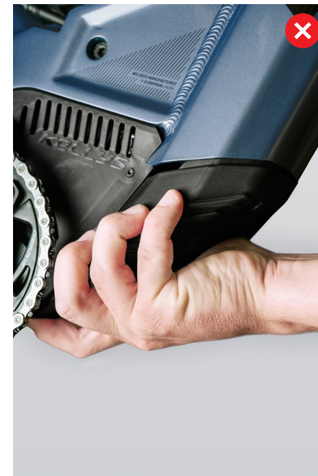
FIGURE 8: CHECK THE BATTERY COVER OVERLAPPING THE ENGINE COVER ON THE RIGHT SIDE (DRIVE SIDE)
