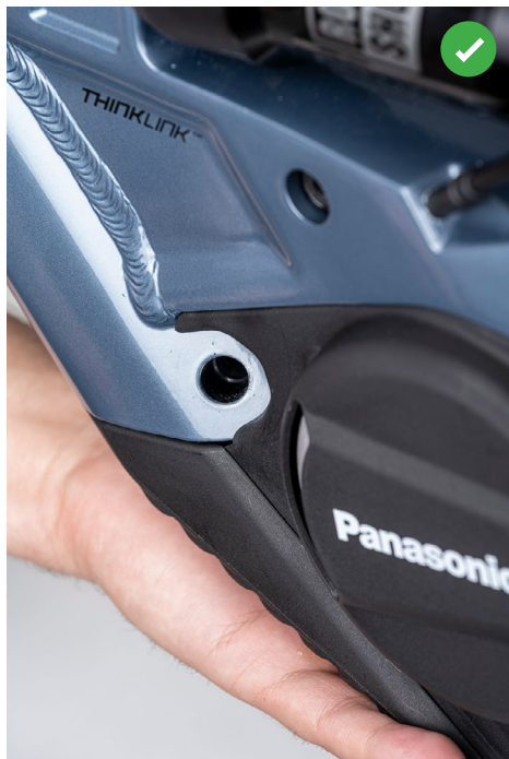
FIGURE 7: CHECK THE BATTERY COVER OVERLAPPING THE ENGINE COVER ON THE LEFT SIDE (NON-DRIVE SIDE)
