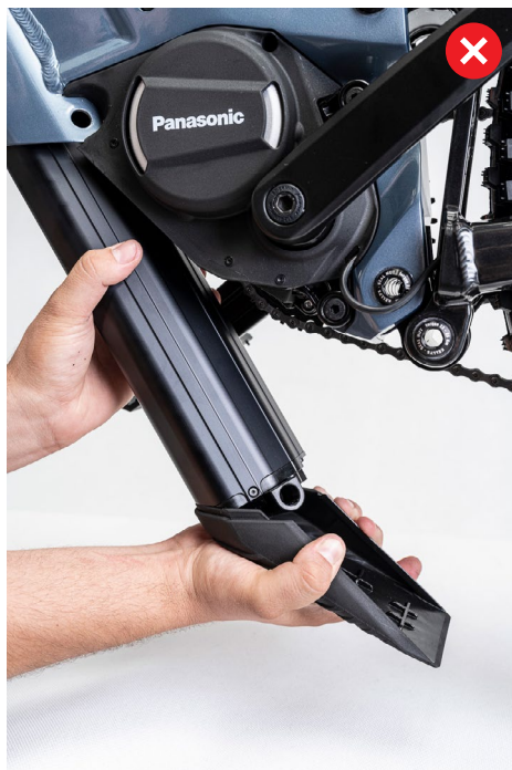
FIGURE 5: INCORRECT BATTERY HOLDING
