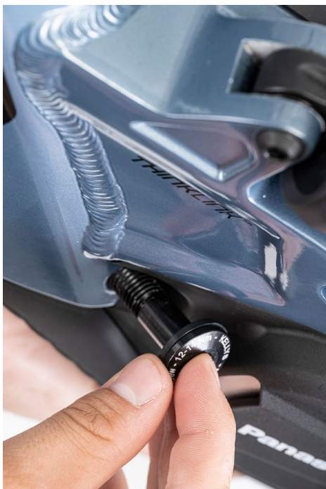
FIGURE 9: LOOSELY INSERTED SCREW IN THE FRAME
