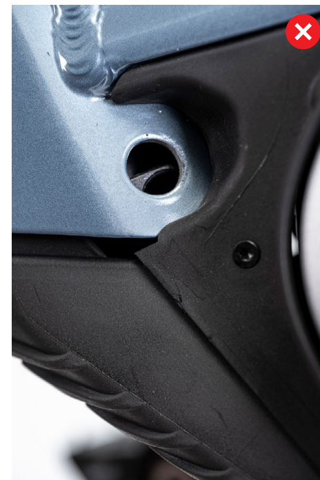
FIGURE 6: CHECK THE HOLE CONCENTRICITY IN THE FRAME AND THE BATTERIES
