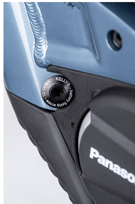
FIGURE 10: SCREW HEAD WITH PRESCRIBED TORQUE
