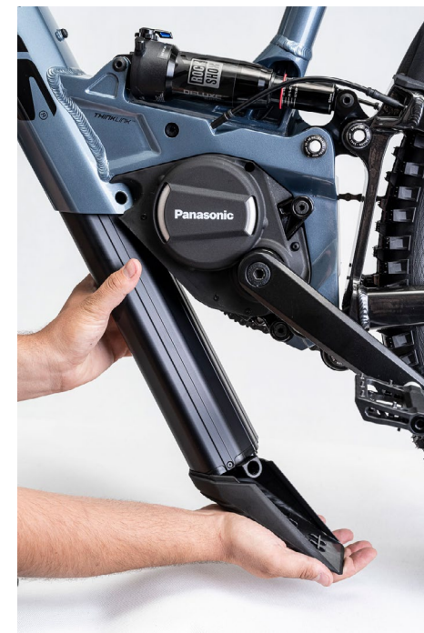
FIGURE 3: CORRECT BATTERY HOLDING DURING REMOVAL
